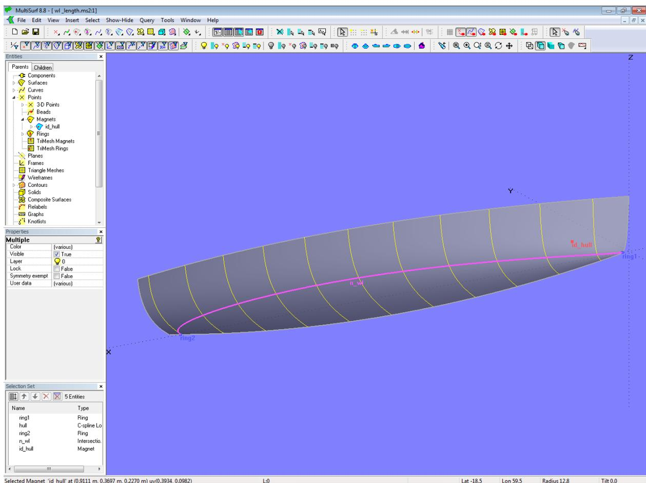
The model shows hull surface “hull”. We want to measure the waterline length.
